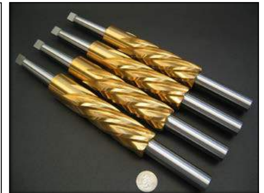
HSS 6-Flute Piloted Finish Reamer, #2 MT shank, 12" OAL Diameter 1.2498" + .0002, - .0000" tolerance with TiN Coating
