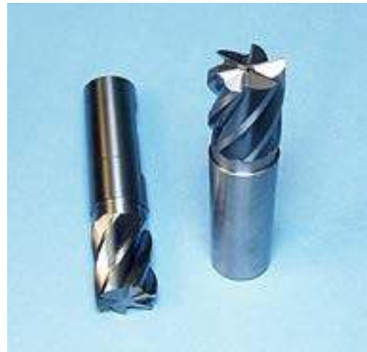
Solid Carbide Special Geometry End Mill
