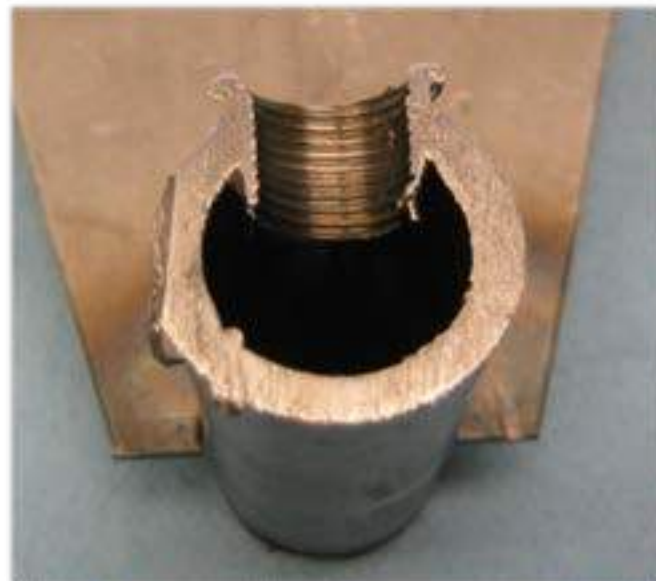
EXAMPLE OF FLOW DRILLING OF NATURAL GAS PIPE FOLLOWED BY FORM TAPPING - CHIPLESS!
