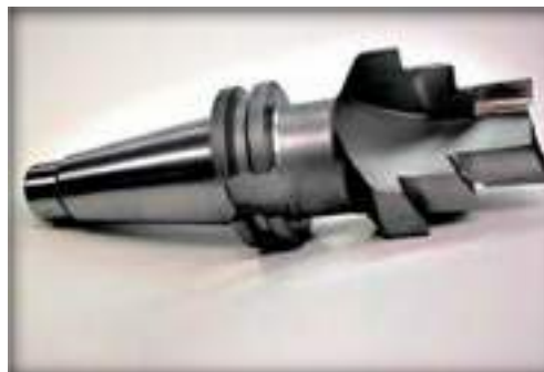
Carbide Tipped Multiple Step Finish Ream and Facing Tool
